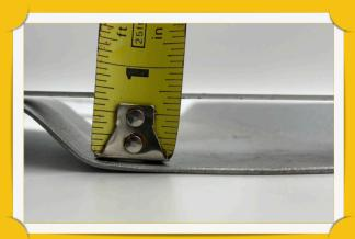
Use a straight edge to measure the height of your container's roof ribs. They should be approximately 3/4 of an inch.
